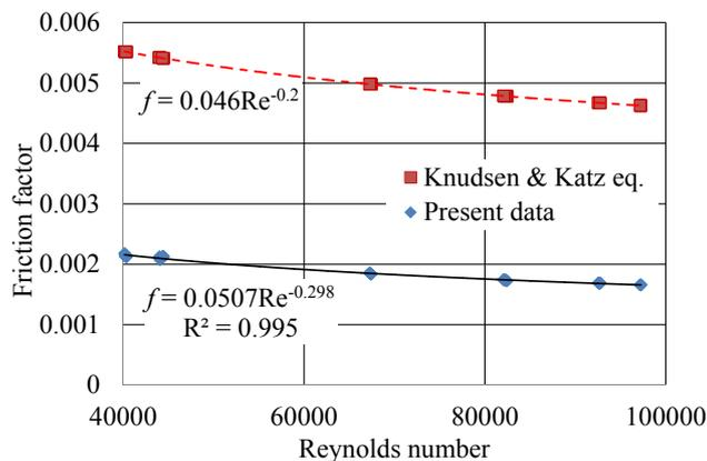
Fig. 4. The friction factor: present experimental data and Eq. (7).
