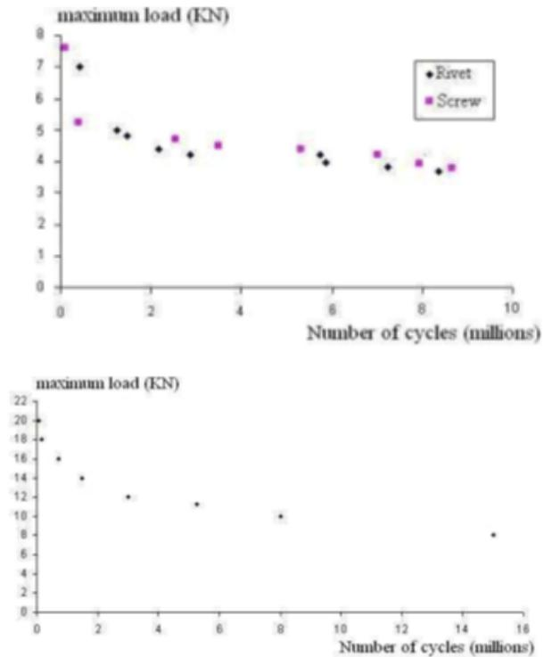
Fig. 9. Wöhler's curves in shear configuration, screwed/riveted joints & bonded joint
