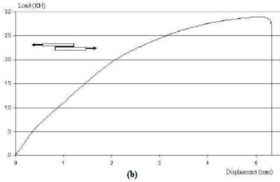
Fig. 7. Static tests for the shear configuration assembled by (a) screw /rivet and by (b) adhesive
