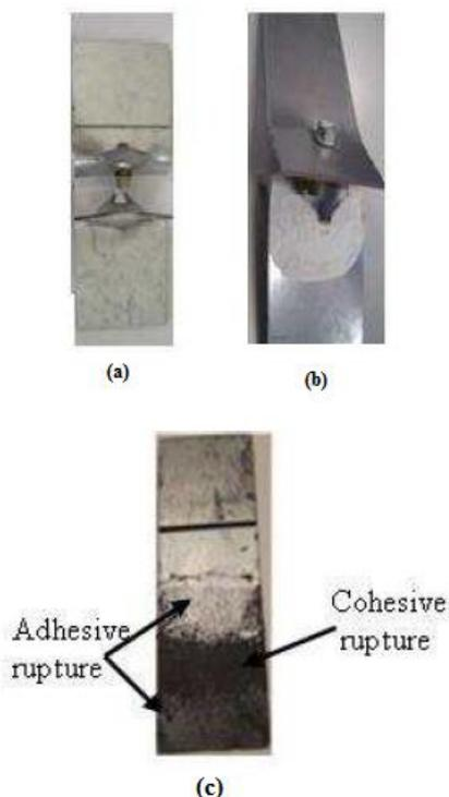
Fig. 11. failure for the joints with shear configuration: riveted joint (a), screwed joint (b), bonded joint (c)
