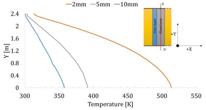
Fig. 6. Temperature profile along the C-C' line inside the curtain wall.
