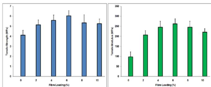
Fig. 5. Effect of CNC loading on (a) mechanical tensile strength and (b) tensile modulus
