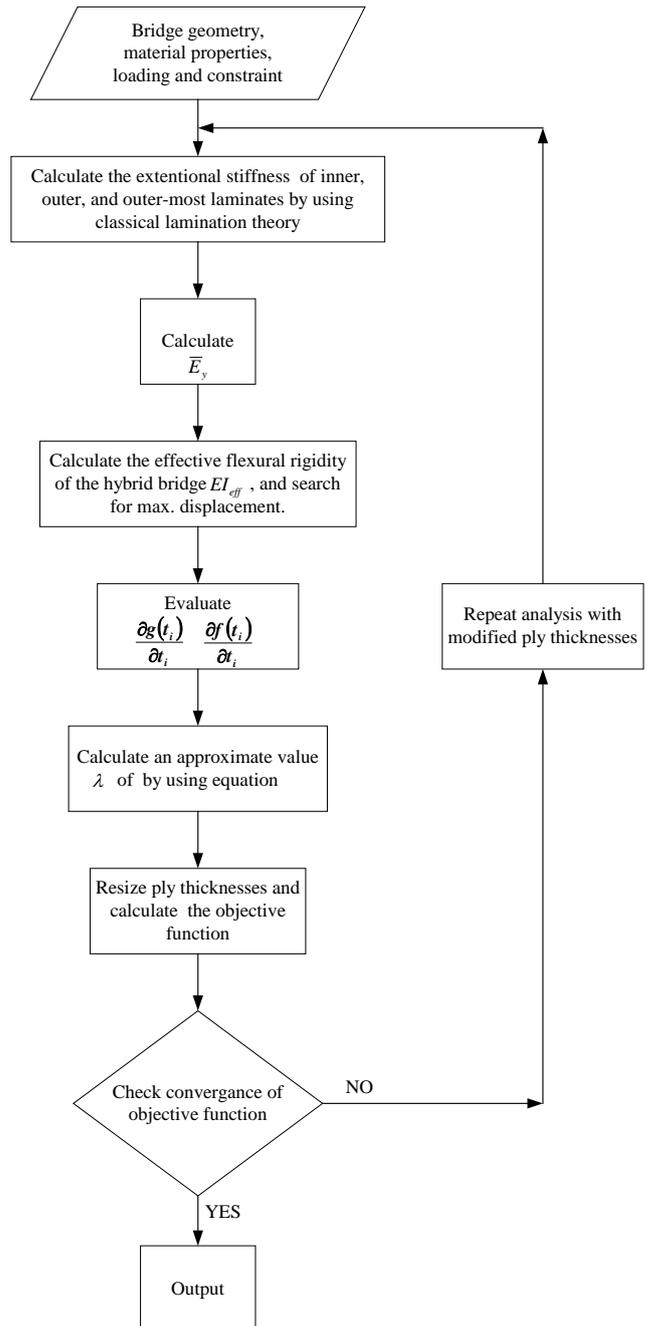
FIGURE 2 FLOW CHART FOR OPTIMIZATION PROCEDURE
