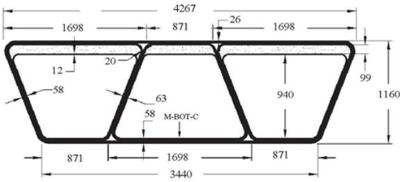
FIGURE 1 CROSS SECTION OF THE HYBRID FRP-CONCRETE SUPERSTRUCTURE (DIMENSION IN MM)
