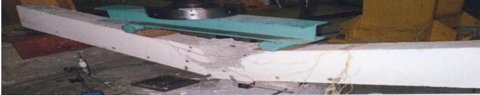
Fig. 4. Failure mode for control beam CB1
