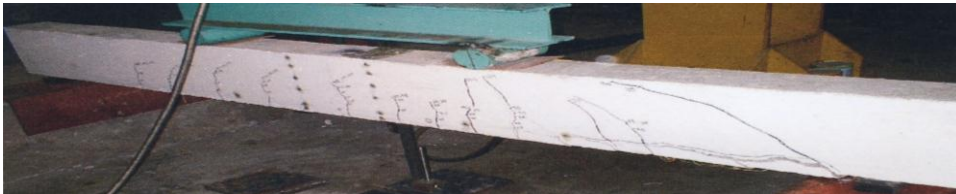
Fig. 6. Failure mode for strengthened beam without end anchorage S-F-0
