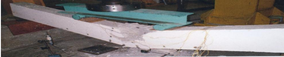
Fig. 4. Failure mode for control beam CB1
