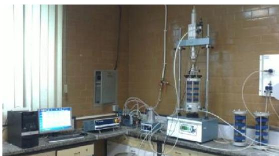
Fig. 3. Cyclic triaxial device set
