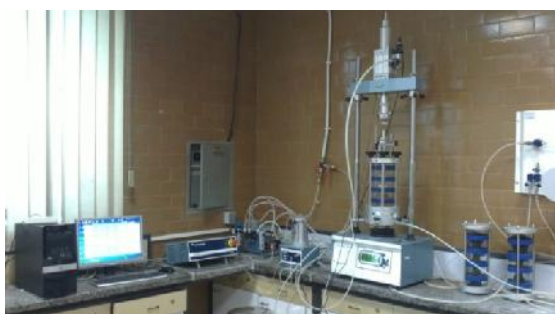
Fig. 3. Cyclic triaxial device set
