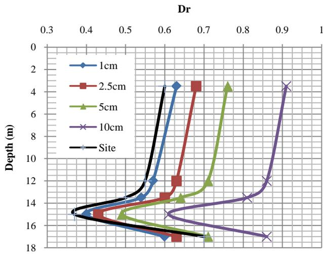
Fig. 2. Changing the relative density by depth to compare the site investigations with model results in 3m spacing of micropiles and for 4 boundary displacement.
