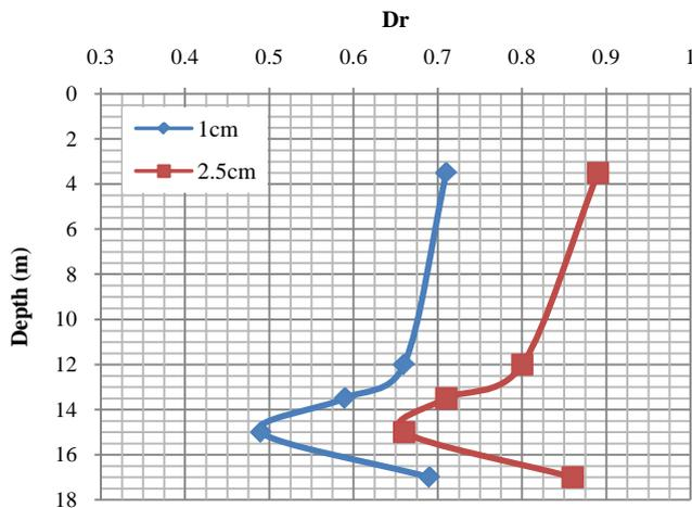
Fig. 4. Changing the relative density by depth in 0.8m spacing of micropiles and for 2 boundary displacement.
