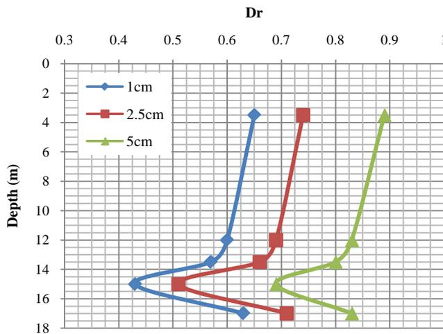
Fig. 3. Changing the relative density by depth in 1.6m spacing of micropiles and for 3 boundary displacement.
