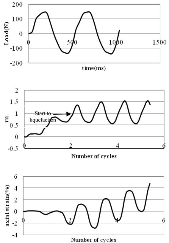
Fig.5. Behavior of Unreinforced sand during cyclic tests (Unreinforced sand,  $P'_0=100\text{kPa}$ ,  $\text{CSR}=0.19$ ,  $\text{Dr}=0.30$ )
