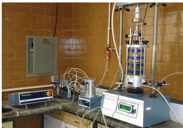
Fig. 3. An overall view of the cyclic triaxial apparatus.
