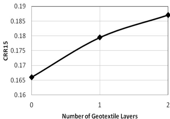
Fig. 9. Effect of geotextile layers on the cyclic resistance ratio (CRR)
