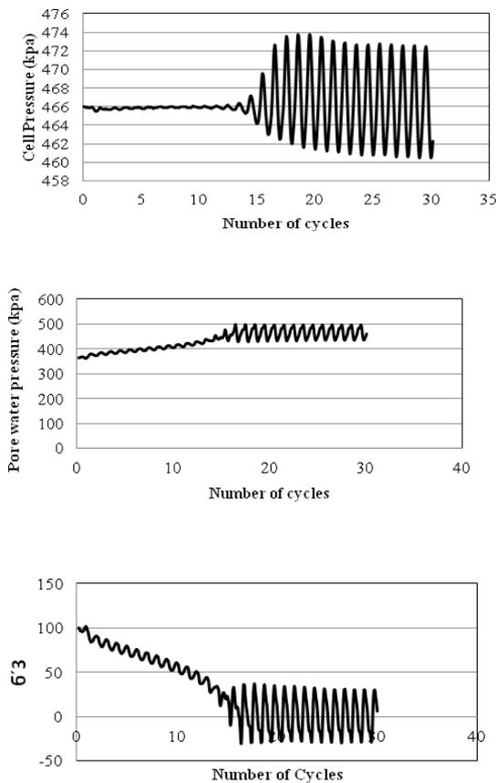
Fig. 4. Changes in pressures during cyclic tests ( $P'_0=100\text{kPa}$ ,  $\text{CSR}=0.16$ ,  $\text{Dr}=0.30$ )
