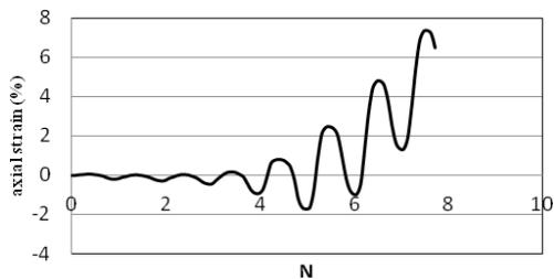
Fig. 6. Behavior of reinforced sand during cyclic tests
