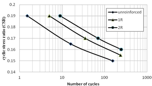
Fig. 8. Effect of reinforcement on the liquefaction of soil.
